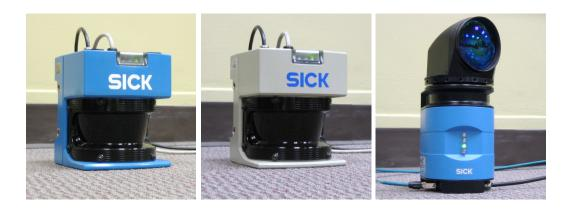
Figure 1: The Sick LIDAR Matlab/C++ Toolbox supports both the LMS 2xx and LD families of Sick LIDARs. Pictured are a few of the Sick LIDARs used to explicitly test the toolbox: (Left) A Sick LMS 200–30106 (Center) A Sick LMS 291–S05. (Right) A Sick LD–LRS 1000.
